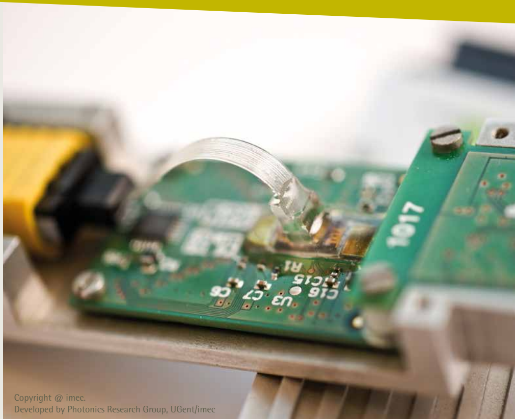
Opto-electronic transceiver for "Fiber to the home" applications
