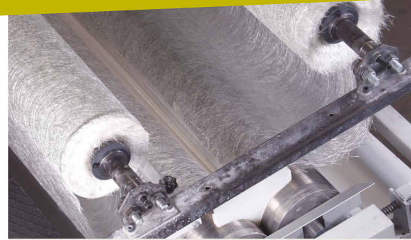
Photo 1: Newly developed impregnator machine which can impregnate several glass mats at the same time, having only a very small quantity of matrix "work in progress". Using a unique texture surface on the pressure rolls, the equipment has a production capacity of 400 m 2 per hour, and more.
