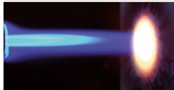
Photo 2: The vubonite material is completely fireproof and incombustible.
